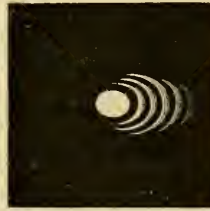
Fig. 69.—Appearance of same object when object-glass is out of adjustment.
